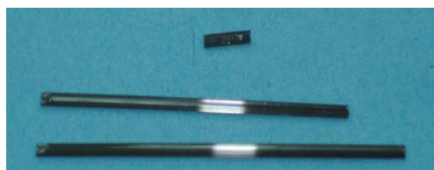
Fig. 2. Macroscopic view of optical fiber bundles (2.5 mm) with damaged and fractured places ( \text{Nd}^{3+} : YAG, 4.1 kW, 14J, 2180 J/cm 2 ).
